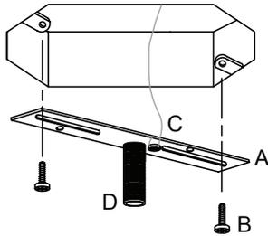
1. Carefully unpack parts. Fasten Mounting Strap (A) to Outlet box with Machine Screws (B).
